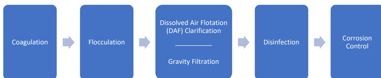
Figure 2-5. Overview of Proposed WJWW Plant Treatment Process
