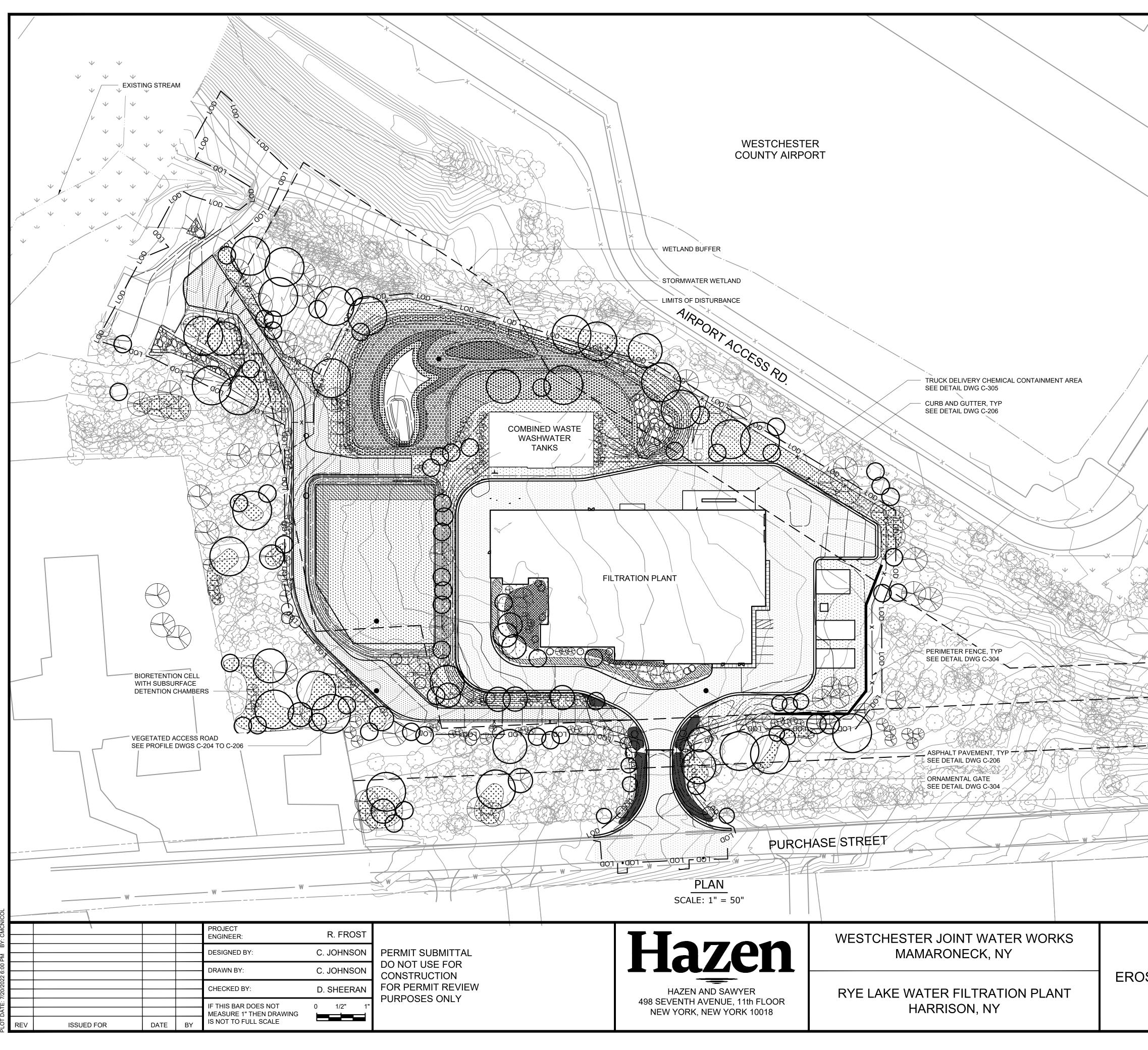
EROSION AND SEDIMENT CONTROL - PHASE 4 - FINAL GRADING AND PAVING
