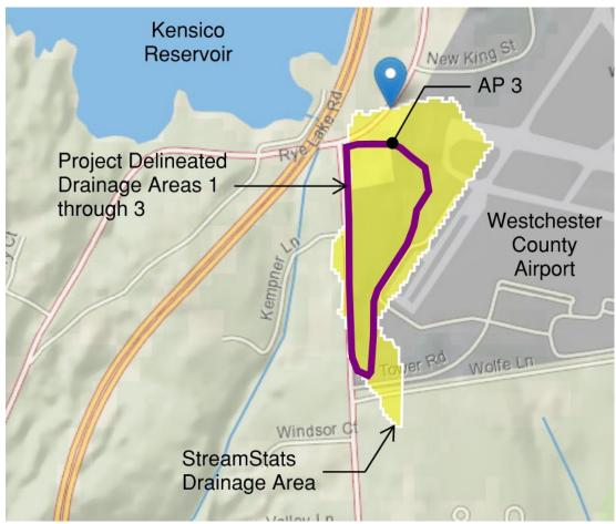
Figure 5-1 - StreamStats Drainage Area
