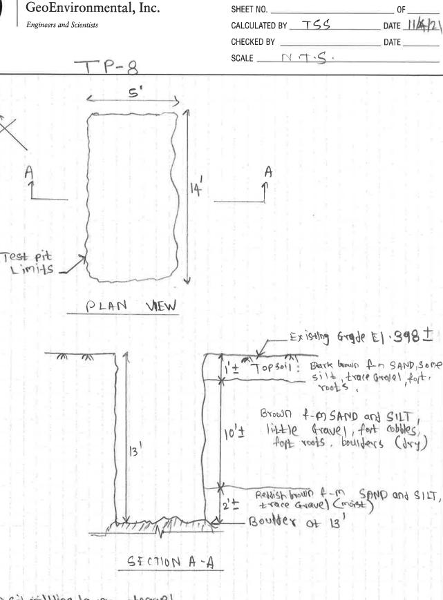
1. No soil nottling layer observed 2. No Groundwater observed
