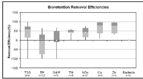
Figure 5. Bioretention Removal Efficiencies
