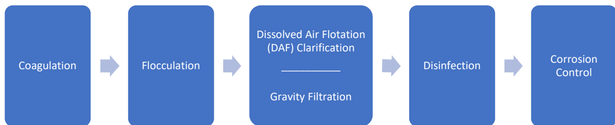
Figure 1-5. Overview of Proposed WJWW Plant Treatment Process
