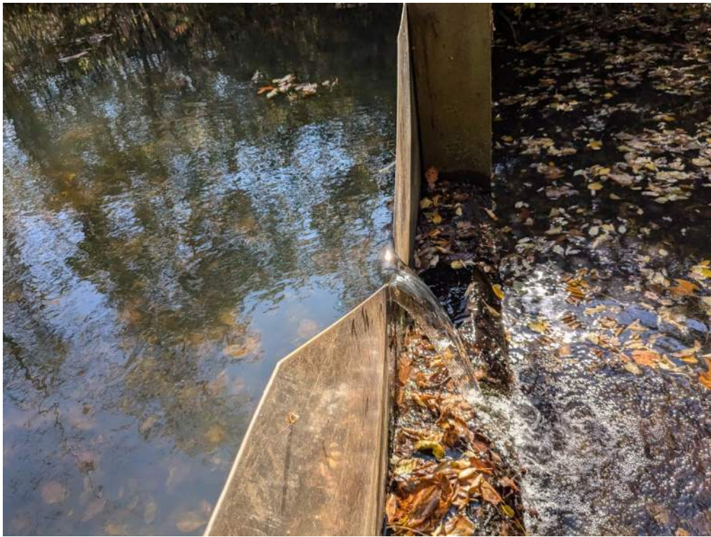
Photo 2. Outflow over 120-degree v-notch weir
